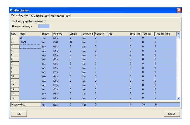
Every table line includes a phone number prefix (of variable length) and other parameters. The parameters define SmartGate's behavior in case the beginning of the dialed number matches this prefix on the same table row. The table contains 120 rows for up to 120 different prefixes.
